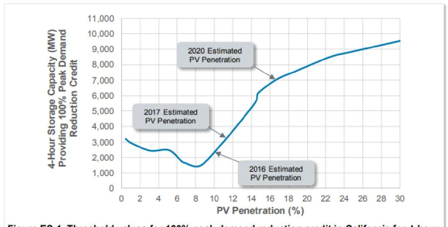
Figure ES-1. Threshold values for 100% peak demand reduction credit in California for 4-hour energy storage in 2020 (assuming a peak demand of 54 GW)
