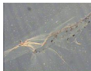
Figure 1. A fiber that formed overnight on a thin film of xSIBS.
