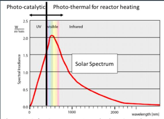
Figure Y: Solar Spectrum. A method we intend to use to reduce the reactor heating load is to take advantage of the entire solar spectrum to provide photocatalytic energy to drive the reaction and photothermal energy to heat the reactor.
