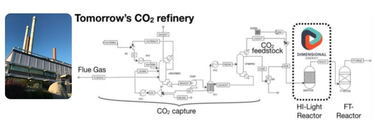
Figure 1.4 Schematic illustration of the 'CO2 refinery'. The HI-Light reactor developed at Dimensional Energy is integrated with upstream CO2 capture and downstream syngas conversion in a Fischer-Tropsch (FT) reactor to form higher hydrocarbon products.
