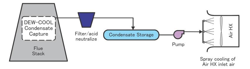
DEW-COOL: Deferred Evaporation of Water Condensate Obtained Locally
