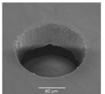
Ultrafast, femtosecond pulse lasers (right) will eliminate machining defects in fuel injectors.
