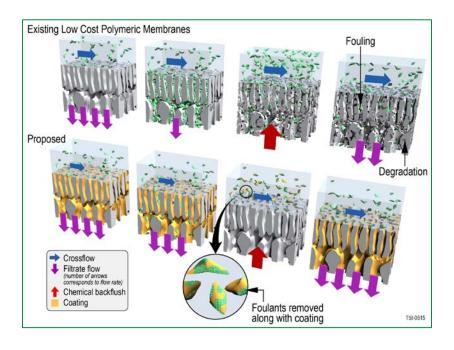
Protective coating materials for high-performance membranes, for pulp and paper industry.
