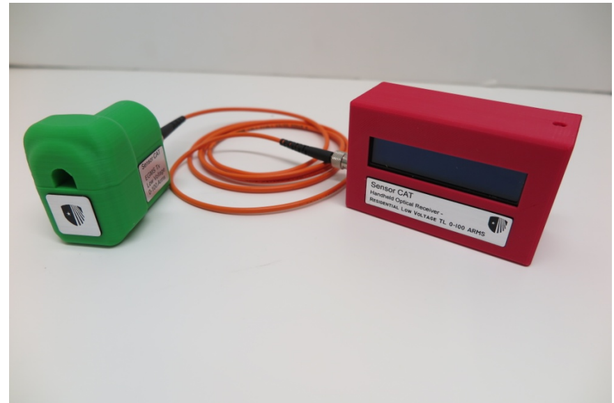
Experimental sensor for “underground” power lines with optical fiber readout unit.
