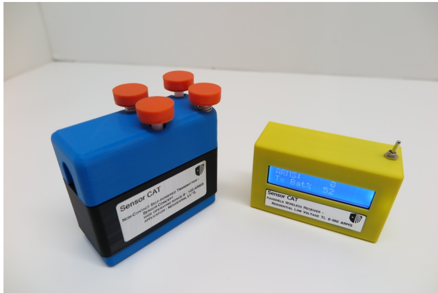
Experimental sensor for “on pole” power lines with wireless readout unit.
