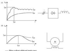
— Motor without additional inertia mass --- Motor with additional inertia mass
