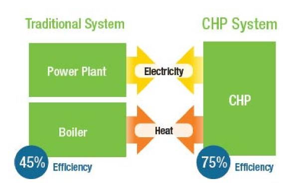
CHP is efficient, because the heat and power are generated closer to where they are used.
