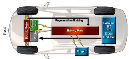
Battery Electric Vehicle (BEV) = EREV – Engine – Generator – Fuel Tank
