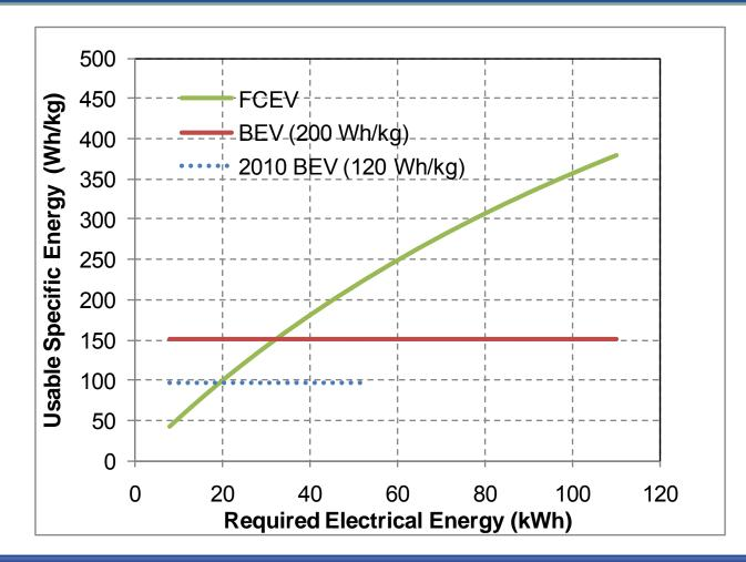
It is the fundamental dependence of the specific energy on the amount of electricity required which determines the applicability of these systems in vehicles of various size and range.
