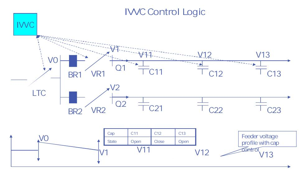
Feeder Voltage Profile With CVR Contrl in IVVC
