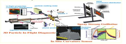
Fig. 1: Sensor set-up to explore process capabilities.
