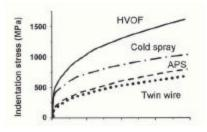
Fig. 1. Stress-strain curves for Ni-5%Al
