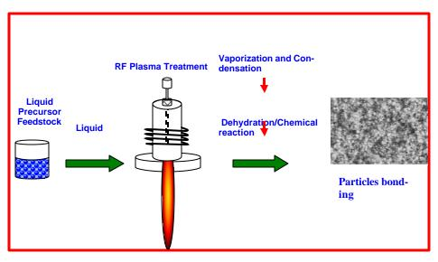
Fig. 2: Schematic of precursor plasma spraying process.
