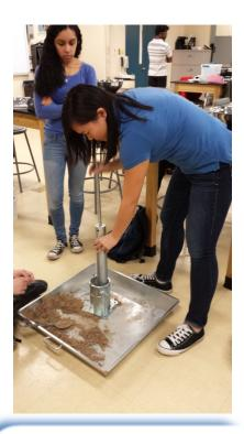
Gabby and Emily working on a proctor compaction test in lab.
